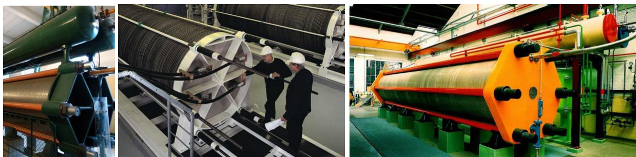
Figure 2: Large scale Alkaline electrolyzers
